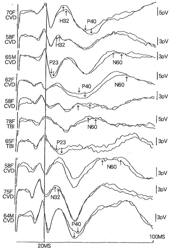
Fig. 6 Examples of wave-forms which showed significant changes of MSEP in the same subject. SSEP was reproducible but MSEP changed according to the arousal level and habituation.
