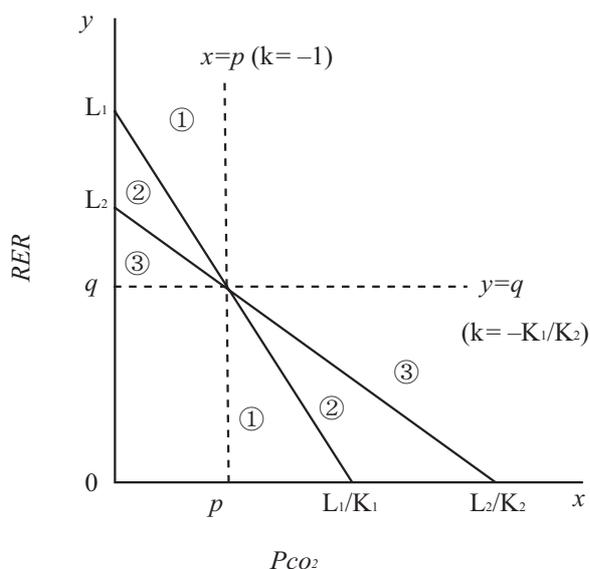
**Fig.3** The third regression line in another condition can be written as  $y = -(K_1 + kK_2)/(1 + k)x + (L_1 + kL_2)/(1 + k)$  with a constant  $k$ . For the regions ①, ② and ③, see Table 1.
